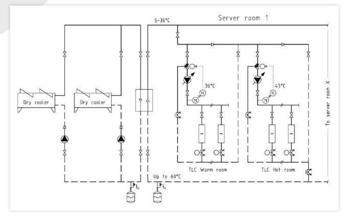
Image 12 Free Cooling based Temperature Chaining by Tebodin Bilfinger
