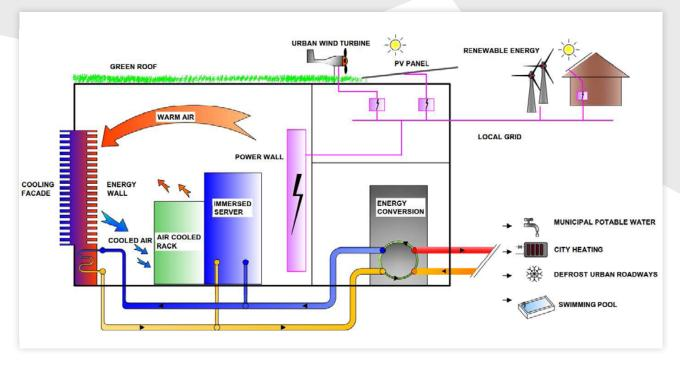
Image 14 Concept for a purpose built micro edge datacentre by Tebodin Bilfinger
