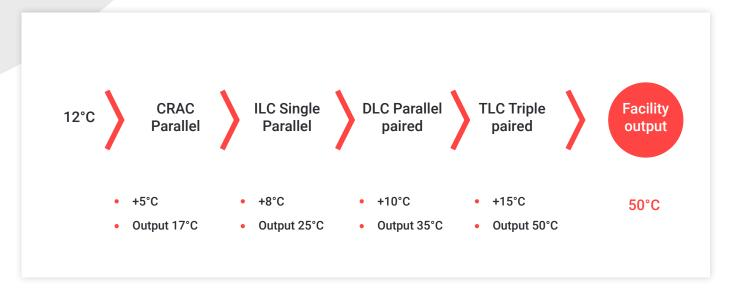
Image 6 Temperature chaining principle
