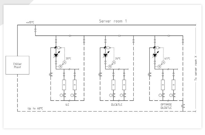
Image 11 Chiller based Temperature Chaining by Tebodin Bilfinger
