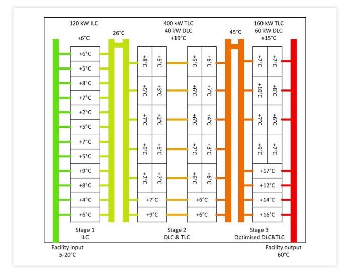
Image 8 Open Circuit heat reuse schematic (temperatures are random)
