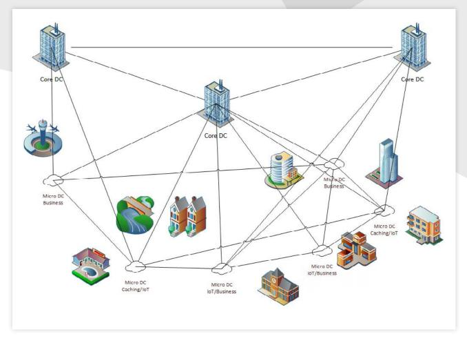
Image 13 Datacentre environment consisting of core datacentres and edge nodes
